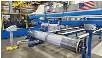
ASC Machine Tools, Inc. designs and manufactures seaming tables and drum winding stations for the production of roll-up doors.
