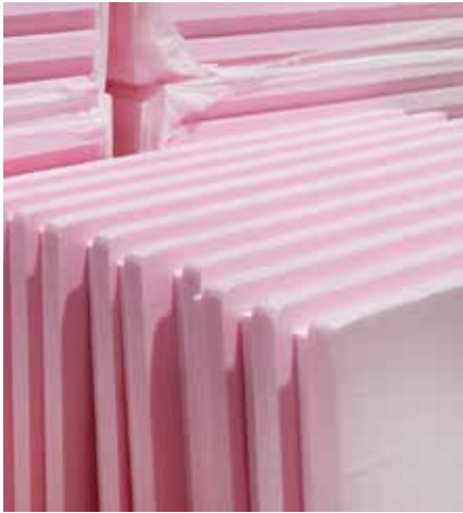
Form board (rigid foam) insulation.
