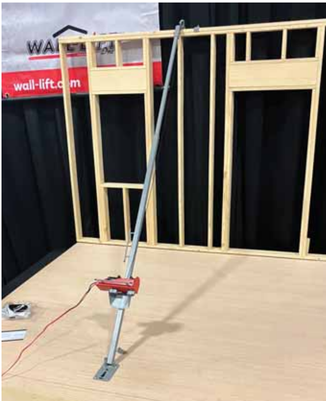
Wall-Lift is a powered hoist system for lifting walls. Each unit can lift 440 pounds. A small but powered demonstration unit was on display.
