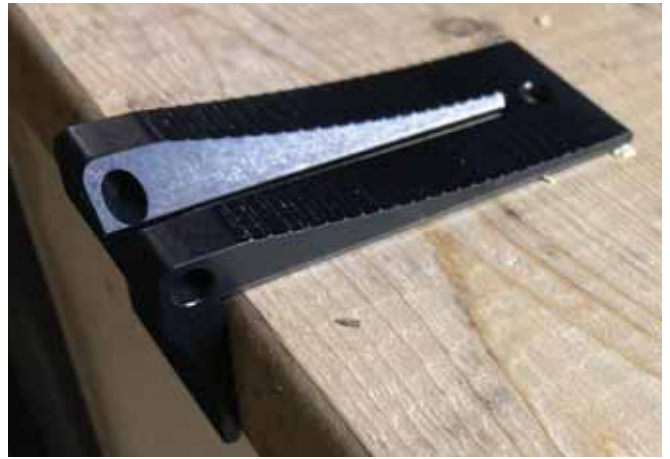
Above and bottom left are photos of a saddle square. Bottom right is a marking gage.
