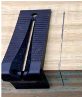
Above and bottom left are photos of a saddle square. Bottom right is a marking gage.
