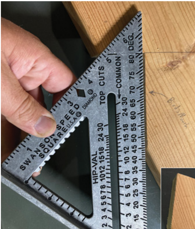
Aligning the heel cut, above. At right is a jig that you can make yourself.
