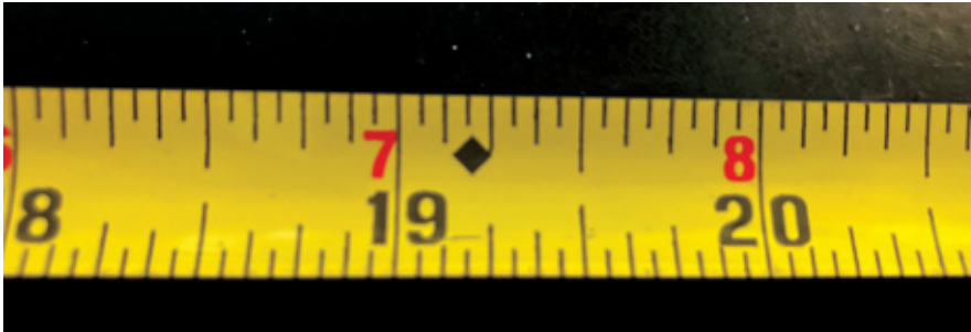
Above, some tapes have a black diamond at 19 3/16" related to truss installation. Below, you can see two quality brands that agree with each other, and a cheap tape that's off. Top right: Use the housing length and stop trying to bend the tape into corners.
