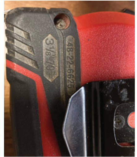
Above, some tapes have a black diamond at 19 3/16" related to truss installation. Below, you can see two quality brands that agree with each other, and a cheap tape that's off. Top right: Use the housing length and stop trying to bend the tape into corners.
