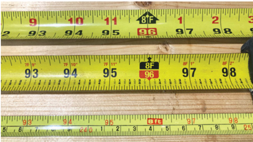
Above, some tapes have a black diamond at 19 3/16" related to truss installation. Below, you can see two quality brands that agree with each other, and a cheap tape that's off. Top right: Use the housing length and stop trying to bend the tape into corners.
