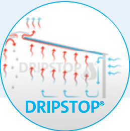
Effective condensation control requires good building ventilation
