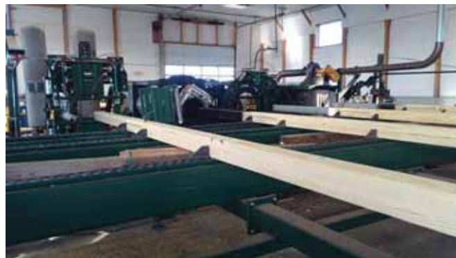
The Super-Winder machine yields 45 posts per hour.
