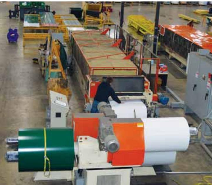
(LEFT) Uncoiling and rollforming at Hixwood Metal in Stanley, WI. PHOTO COURTESY OF SHARON THATCHER
