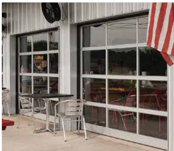
Framed glass doors give buildings a contemporary look. Since the glass is much heavier than other materials, it puts more limitations on the operators that can be used.
