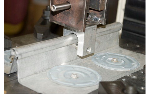
S-5! Holding Strength Test
