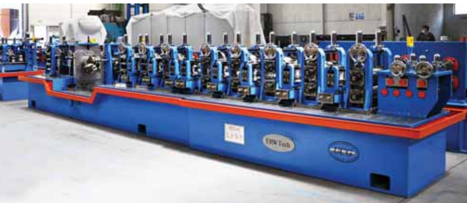
A new UCG/ERW Tech Carport Tube Mill will come with all the necessary components and was created specifically for the carport industry. This machine is capable of forming whatever size carport framing is needed. COURTESY OF UCG/ERW.
