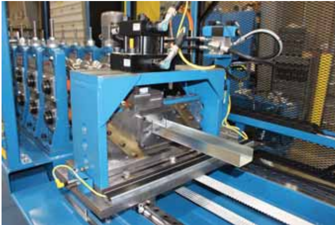
An ASC Machine roll-forming machine produces U channel, which is used for framing. PHOTO COURTESY OF ASC MACHINE TOOLS
