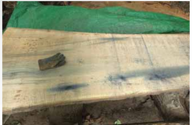
Iron stains in red oak. In this case, bits of steel in the tree caused staining throughout the harvested wood. COURTESY OF WOODWEB.COM
