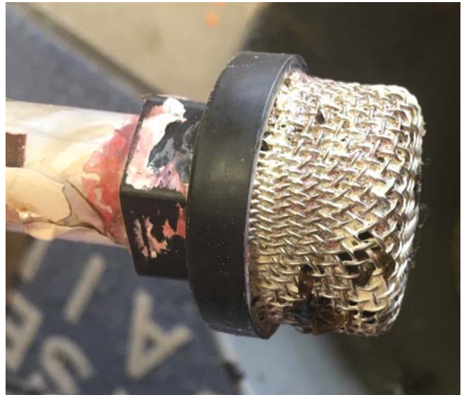
Clogged pick-up tube filter.
