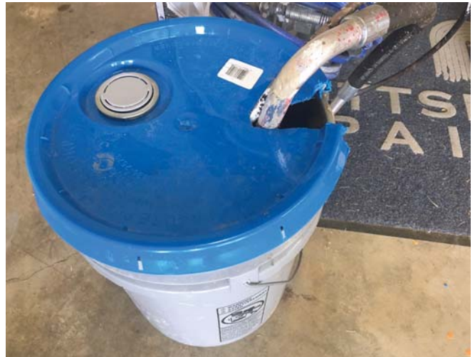
Place the pick-up tube through a “V” cut from an old lid to decrease air exposure and reduce the amount of paint drying in the pail.
