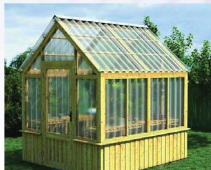
Corrugated panels must always be installed on the roof so ribs run vertically. Horizontal supports should be no further than 36" apart. PHOTO COURTESY ONDULINE (TUFTEX).
