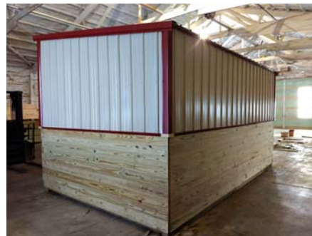
Ideal for animal confinement, Mid Michigan Structures [(231) 825-0382] builds its shelters with kick walls built from treated 2x6 tongue and groove lumber. Buyers often use them to shelter horses, pigs and cows — even alpacas and deer. PHOTOS COURTESY OF MID-MICHIGAN BARN
