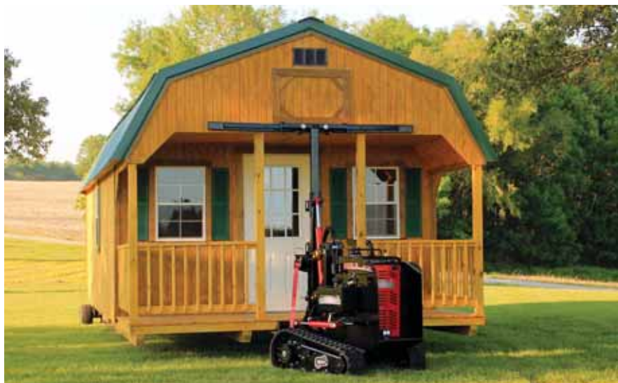
The 727T Mule is Cardinal Manufacturing's most powerful shed mover. It's equipped with an electronic fuel-injected 37HP Vanguard engine.
