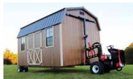
The hydraulic T-bar helps stabilize the shed while being moved into position. PHOTO CREDITS: CARDINAL MANUFACTURING LLC
