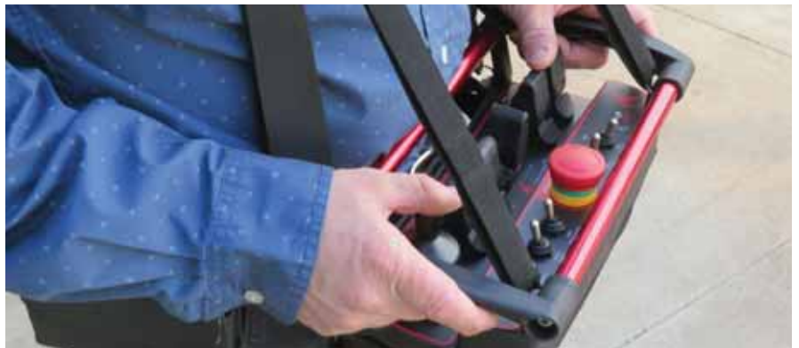
The optional wireless remote control gives the Mule operator maximum visibility while maneuvering the shed into place. PHOTO CREDIT: CARDINAL MANUFACTURING LLC
